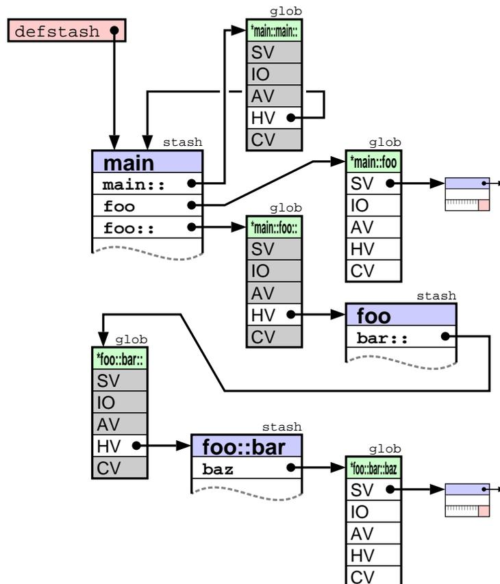
All resolution of qualified names starts with the stash pointed to by the defstash variable. Nested name spaces are implemented by a stash entry with a key ending in "::". The entry for "main::" ensures that defstash is also known as "main" package (and has the side-effect that the "main::main::main" package is defstash too.) Unqualified names are resolved starting at curstash or curcop->cop\_stash which are influenced by the package declaration in Perl.
