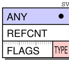
It contains a pointer (ANY) to more data, which in this case is always NULL. All the subtypes are implemented by attaching additional data to the ANY pointer.
