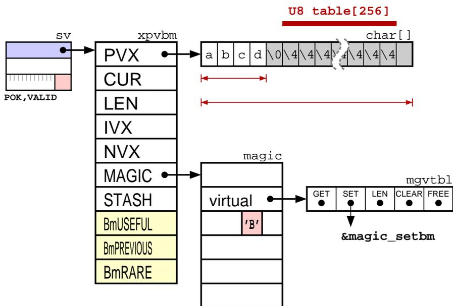
The extra *SvPVBM* information and the character distance table is only valid when the **VALID** flag is on. A magic structure with the sole purpose of turning off the **VALID** flag on assignment, is always attached to a *valid* *SvPVBM*.
