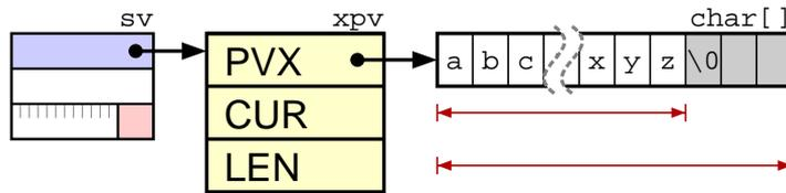
The POK flag indicates that the string pointed to by PVX contains a valid string value. If the POK flag is off and the ROK flag is turned on, then the PVX field is used as a pointer to an SV (see SvRV below) and CUR/LEN is unused. An SvPV with both the POK and ROK flags turned off represents *undef*. The PVX pointer can also be NULL when POK is off and no string storage has been allocated.
