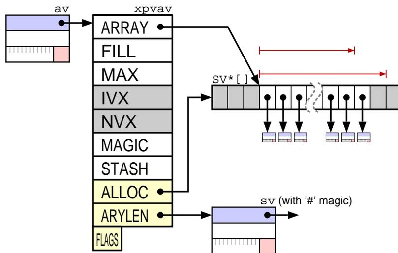
The array pointed to by ARRAY contains pointers to any of the SvNULL subtypes. Usually ALLOC and ARRAY both point to the start of the allocated array. The use of two pointers is similar to the OOK hack described above. The shift operation can be implemented efficiently by just adjusting the ARRAY pointer (and FILL/MAX). Similarly, the pop just involves decrementing the FILL count.
