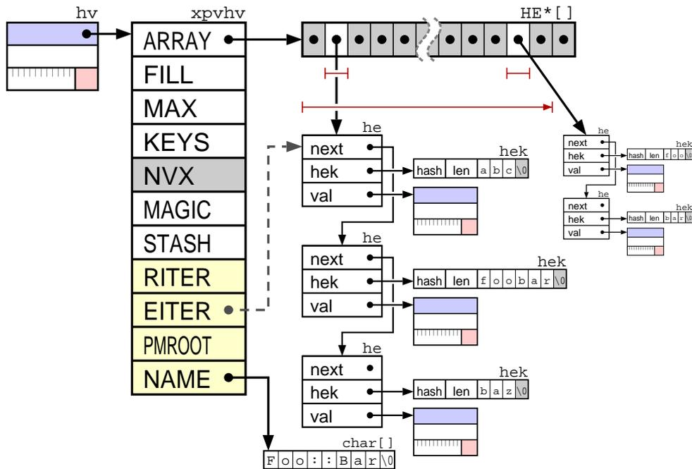
In a perfect hash both KEYS and FILL are the same value. This means than all HEs can be located directly from the pointer in the ARRAY (and all the he->next pointers are NULL).
