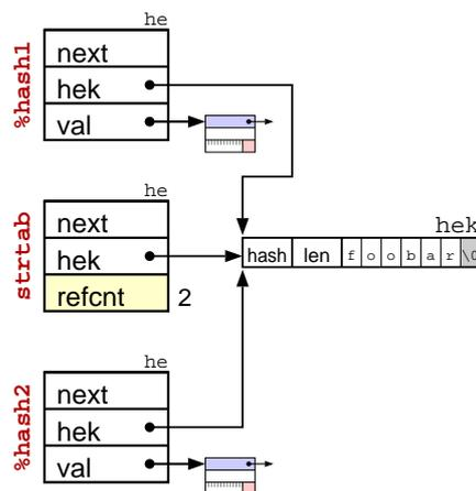
What is special with the `strtab` hash is that the `val` field of the HE structs is used as a reference counter for the HEK. The counter is incremented when new hashes link up this HEK and decremented when the key is removed from the hashes. When the reference count reach 0, the HEK (and corresponding HE) is removed from `strtab` and the storage is freed.
