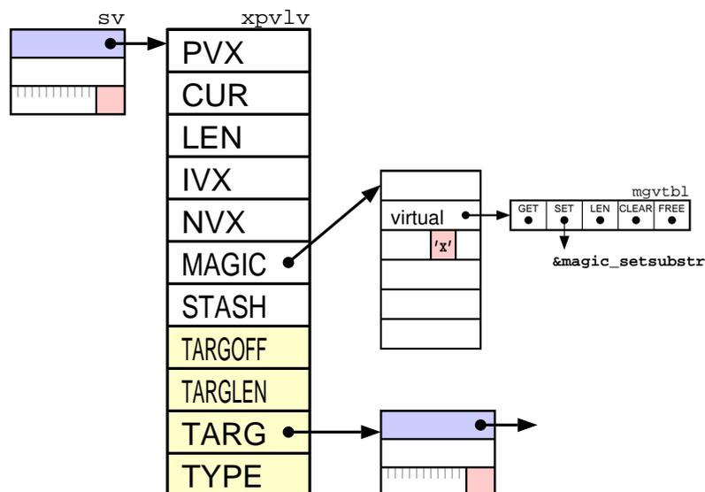
When assignment to an SvPVLV type occurs, then the value to be assigned is first copied into the SvPVLV itself (and affects the PVX, IVX or NVX). After this the magic SET method is invoked, which will update the TARG accordingly.
